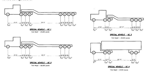
OS/OW applications of Standard Vehicles that cross bridges are reviewed by KDOT staff for approval. Non-Standard Vehicles that cross a bridge will require an individual structural evaluation, which will require additional coordination with KDOT staff. Vehicles are considered to be Non-Standard if:
